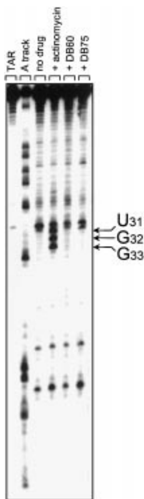
Figure 7. Cleavage of the TAR RNA by the \text{Fe}^{\text{II}} complex of bleomycin A2 (500 \mu\text{M} ) in the absence and presence of actinomycin (10 \mu\text{M} ) or the diphenylfuran derivatives DB75 and DB60 (20 \mu\text{M} each). Actinomycin-induced cleavage sites are pointed out by the arrows. Other details as for Figure 6.
